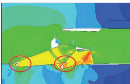
FEA shows how the front and back ferrule grip the tubing on a medium-pressure Swagelok tube fitting rated for use with SAF 2507 tubing.
